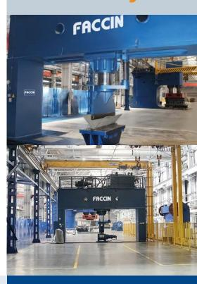
Faccin's 3D PPS forming presses are available with different capacities (from 150 to over 5000 metric tonnes) and different sizes (from 2 up to 10 m gap between uprights).
